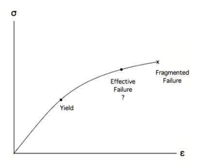
Fig. 6 Failure stress possibilities
