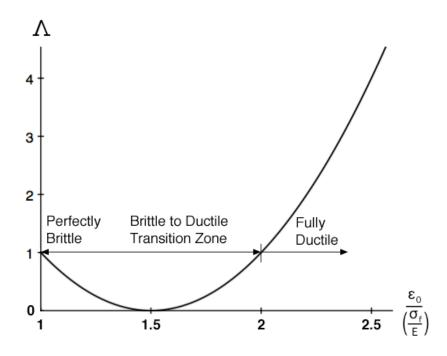
Fig. 9 Energy dominance versus failure strain
