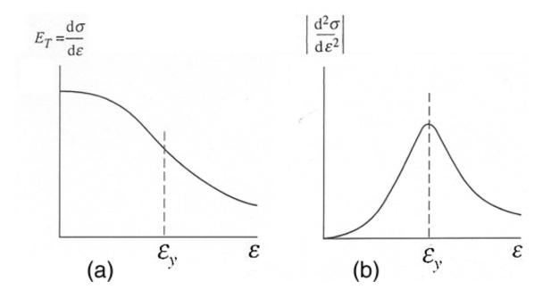
Fig. 2 Derivatives of stress strain curve
